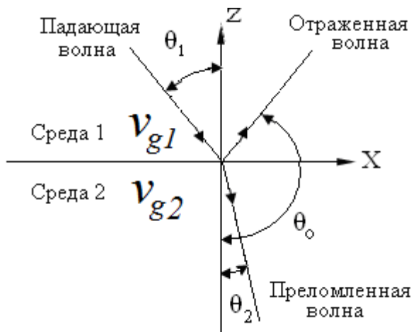
Fig. 3. Reflection and refraction of waves at the two media interface
